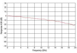
Responsivity measurement of an 80 µm photodiode using the LWP probe and the Agilent Technologies 83420A Lightwave Test Set.
